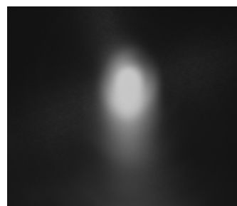
Fig. 3. Near field photograph of the straight waveguide.
