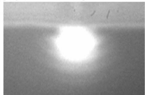
Mode profile of bulk polymer DUV waveguide without water for comparison
